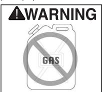
Do not place the compressor next to any flammable liquids or gas! The compressor cylinder head and feed pipe can reach high temperatures and could cause the flammable gas to ignite. Keep work area clear from flammable gas when using the compressor.
